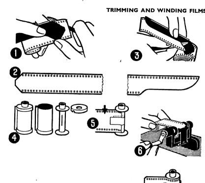
1: The correct trimming of the wedge shaped end (which is attached to the centre spool of the cassette) with standard trimming template. 2: the appearance of the trimmed film, left wedge, right curved cut. 3: Trimming of curved cut with standard template. 4: The cassette, its outer shell, centre spool and cap. 5: How to fix the film to the centre spool. 6: Winding film on to the centre spool with a mechanical winder. 7: Assembling the cassette. 8: Loading film into camera.
