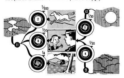
The apertures and shutter speeds on the light value shutter are coupled. With a given light value (e.g., 11), setting a fast speed automatically opens the lens, while stopping down automatically sets a slow speed to keep the exposure constant (left). To alter the exposure for different light conditions, simply change the light value setting (right).
