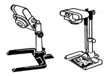
Right: The stereo attachment fitted to the Retina Reflex. An optical system produces two upright pictures side by side with the correct stereo separation.
