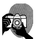
For upright shots, turn the camera through 90° so that it is supported from below with the left hand, the thumb and index finger resting on the focusing ring. The right hand holds the camera steady from above with the index finger on the release button.
