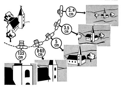
Above: The interchangeable lenses greatly increase the versatility of the Retina Reflex. The wide-angle lens (top) covers a larger angle of view as compared with the standard lens (centre). The telephoto lens, on the other hand, includes a much narrower angle and shows distant subjects larger (bottom).
