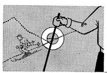
The centre of the viewing screen of the Retina Reflex carries a split image optical rangefinder which shows the incorrectly focused subject in two displaced halves (right). The remainder of the finder field constitutes a ground glass focusing screen. When the subject is accurately focused, it appears sharp on the screen and the two halves of the rangefinder image move together to form a continuous line (above and extreme right).
