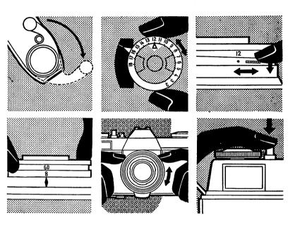
Top left: Wind film by means of rapid winding lever.
