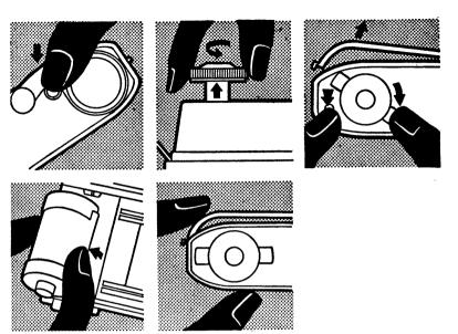
Top left: Press down rewind button on base of camera.
